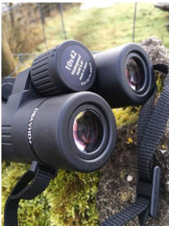
The focus is smooth and precise and is set to 2 turns to go from close focus to infinity. The dioptre adjustment is housed on the focus wheel and once set can be forgotten. I particularly like the locking system as it cannot be adjusted by accident.
